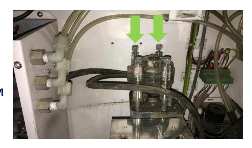
2. REMOVE INSULATION FROM THE TEC BODY TO GAIN ACCESS TO THE TEC MOUNTING BRACKET (2 SCREWS, TB AND SAMPLE TUBING)
